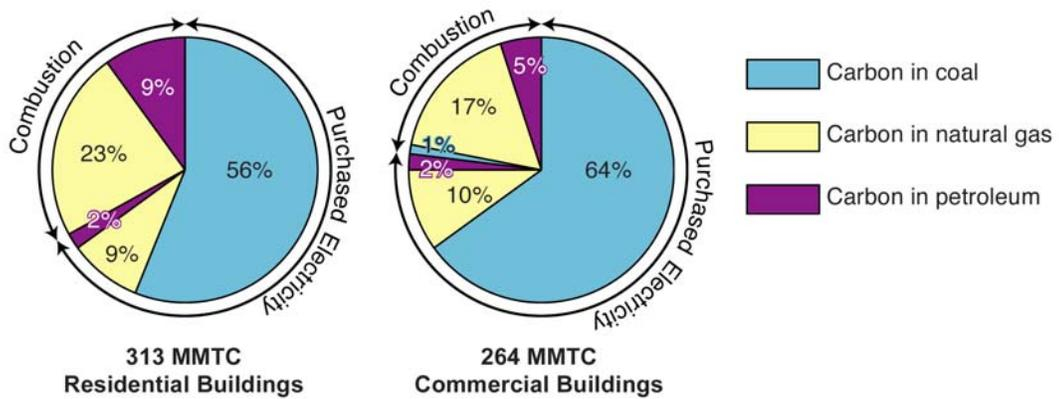
**Figure 2. CO<sub>2</sub> Emissions from U.S. Residential and Commercial Buildings, by Energy Source, 2002**
